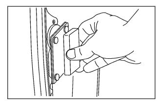
To open the rear portion of a 60/40 door from the outside, pull the handle on the side of the rear door and pull the door toward vou.
